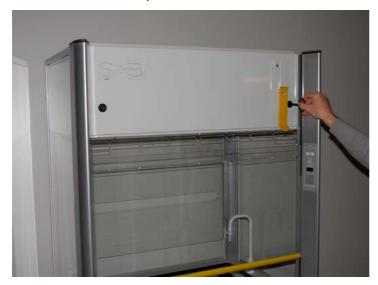
Insert the key and turn both locks through 90deg, which will then release the panel.
