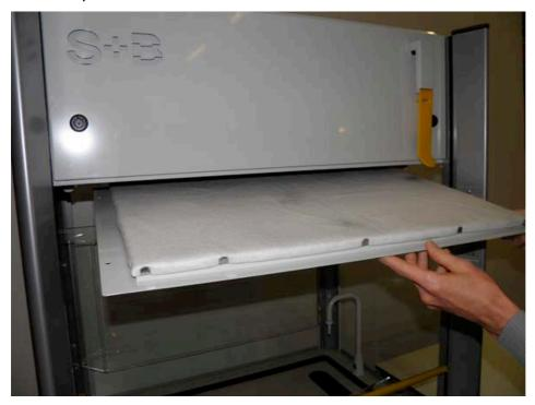
Replace the filter by reversing the process (pre-filters can be obtained from S+B).
